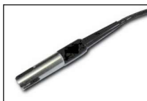
RFT-325 - Measures humidity and temperature. Operating range: -20...+80°C, or -40...+120°C with cable type G. D=8mm, L=35mm
