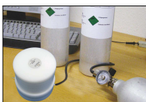
Calibration Kit For DK660 offset calibration includes test gas 400 ppm, regulator and adapter
