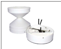
ARG100 Rain Gauge Affordable tipping bucket raingauge. area: 506.7cm 2 sensitivity: 0.2mm
