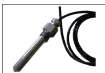
DKRF370-325 - Humidity-/temperature snesor for pressure applications max. 100bar, G3/8" thread, Range -20/+80°C L=100mm, D=13mm
