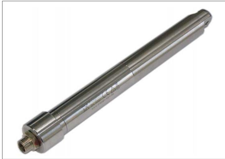
The P-Log3023 measures and records simultaneously pressure and temperature in gases or water. It is available in several different ranges from 1bar to 100 bar. Depending on the type of sensor applied the logger can either log gauge or absolute pressure. An integrated temperature sensor is used for automatic temperature compensation of the pressure reading. Temperature is also recorded as a separate parameter.
